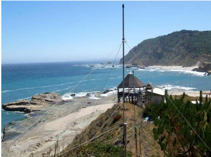
Fig. 2: WERA ocean radar system at Rumena, Chile, (near Concepcion). The system shown operates at 22 MHz and consists of a short array of 8 antennas that receive the signal backscattered from the surface of the ocean.
