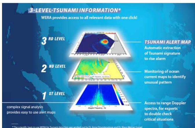
Fig. 3: The WERA tsunami detection software package. It consists of three levels of analysis that can be integrated into any Tsunami Early Warning System. Its application requires a 50 km minimum distance between the coastline and the continental shelf edge.
