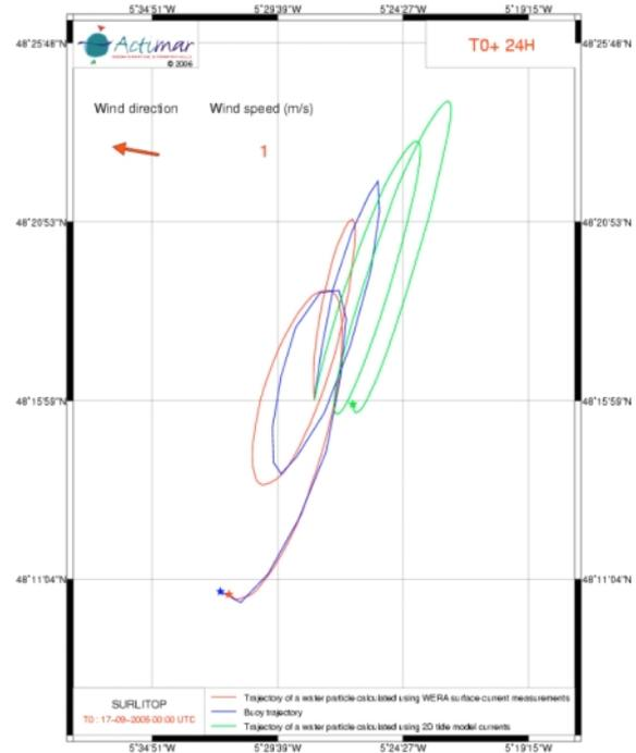
Figure 4. Drifting “person”, real 24 hour trajectory plotted in blue, prediction based on 2D tidal model in green and prediction based on measured data in red
