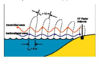
Fig. 1: Principle of operation (Bragg Effect)
