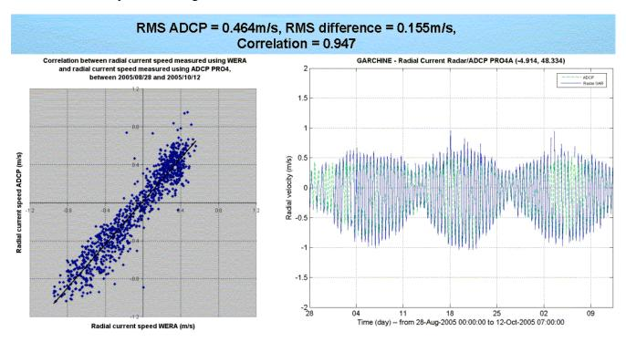
Fig. 7: The current speed measured with WERA was compared with an ADCP measurement For the wave measurements the data were averaged over 1 hour to generate maps same as for the wind direction maps.
