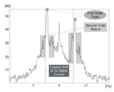
Fig. 2: Typical Spectrum from a WERA system, 1<sup>st</sup> order Bragg lines, shifted slightly off-centre, with superimposed 2<sup>nd</sup> order lines carrying the wave information
