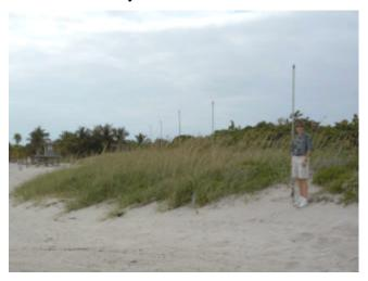
For any WERA site a separation of the transmit and receive antenna arrays of at least 150 m is required. It is preferred to have the linear receive array and the transmit array exact in-line.
