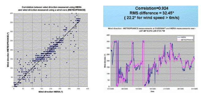
Fig. 10: The WERA measurement of wind direction compared with a wind vane on the island Similar correlation were carried out during various experiments at the Norwegian, Spanish, British and US coast [10, 11, 12].
