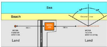
Fig. 3: Typical WERA site geometry
