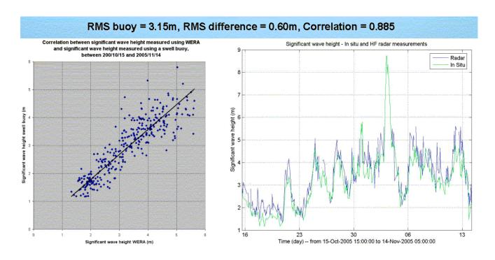
Fig. 10: The WERA measurement of significant wave height compared with a RMS buoy
