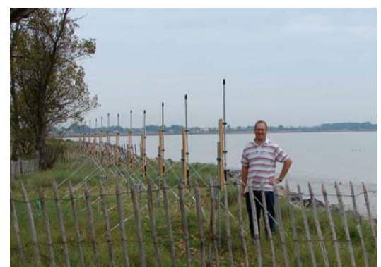
Figures 3: WERA VHF mobile installation in France
