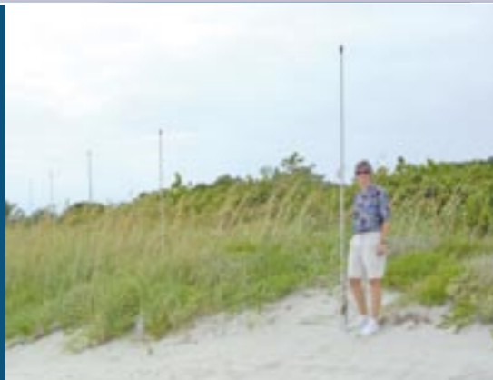
▲ WERA linear antenna array at a public beach on Key Biscayne, USA
