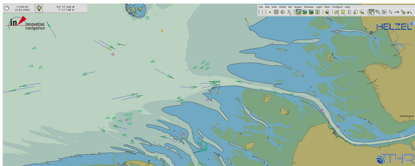
Fig 2: Map with ship tracks generated by WERA on Wangerooge island. The green marked targets are identified by means of AIS. The orange marked targets don't have any identification or have turned off their AIS and thus these targets are visible on the radar monitor only.
