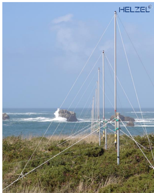
Fig. 1: WERA Antenna Array on the French coast near Brest
